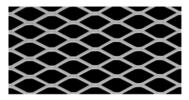
LW Pitch:38.10mmStrand Width:1.91mmSW Pitch:16.48mmThickness:1.20mmWeight:2.23 kg / m2Open Area:77%
